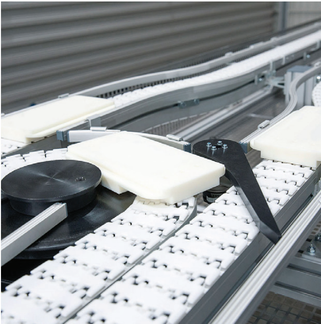
Diversers economically and effectively help control pallet flow on a VersaFlex pallet-handling system.
