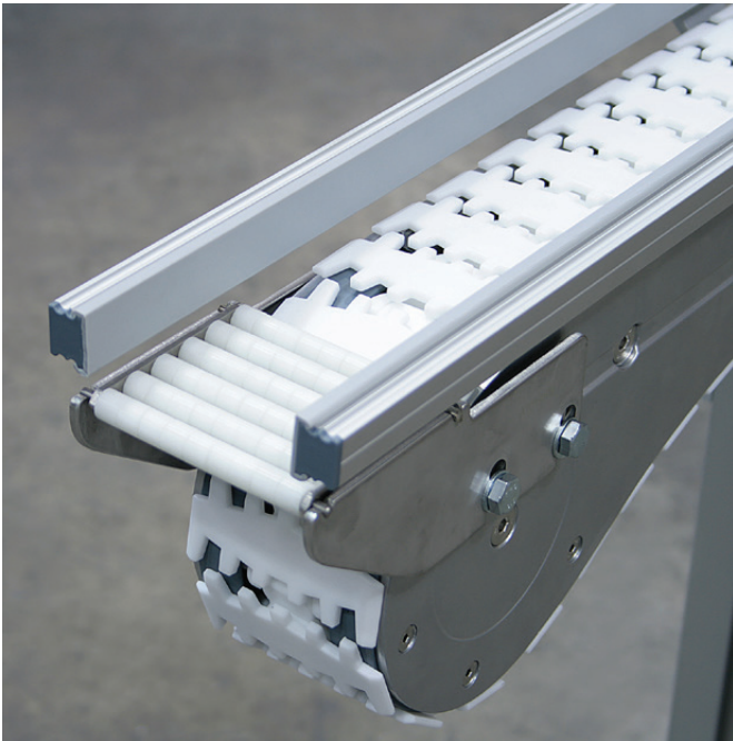
Product transfers, such as the rollers seen on this idler, make it possible to convey products with small footprints between conveyors.
