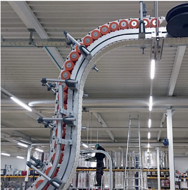
Vertical product conveying is possible for the VersaFlex. In this application guider-rollers above the chain help contain the product.
