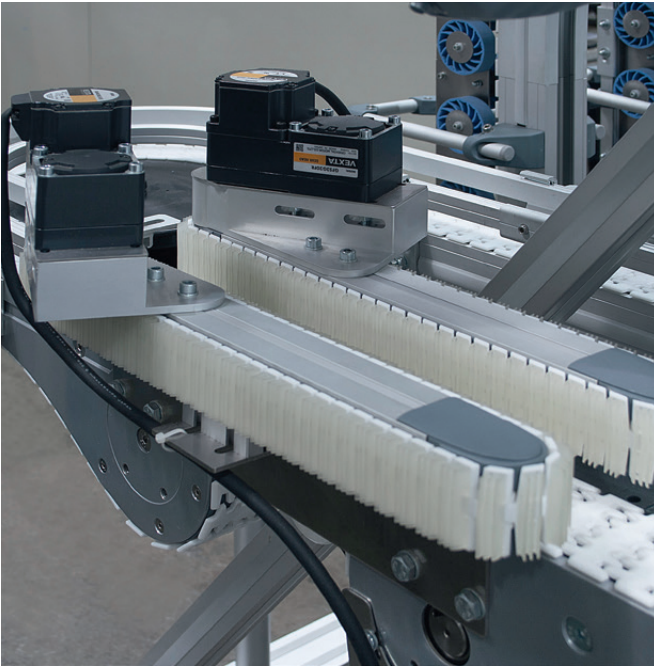
Grip top belting allows for VersaFlex conveyors to be used as side-gridders, to carry the product from one conveyor to the next.
