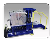
Bowl feeder load systems accommodate a wide range of parts for assembly processes.
