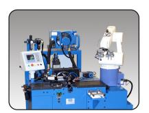
Robotic integration for part loading, unloading and transfer.
