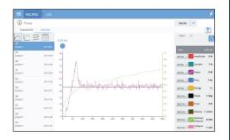
Graphs showing up to 10 weld parameters including energy, power, velocity, distance and force
