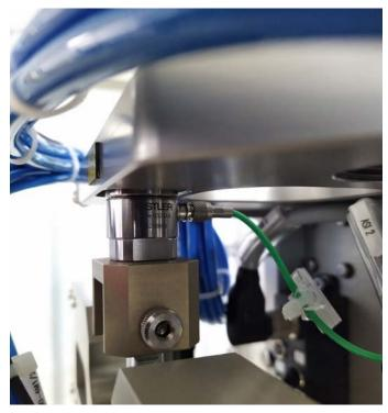
The 9323AA press force sensor from Kistler monitors both the drug insertion step and the reintegration of the actuator module into the auto-injector.
