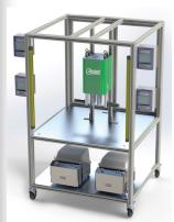
ASG designed an automation cell which allowed the entire assembly process to take place in one location. More importantly, it automated the adhesive application. The ASG Automation solution utilized a fully contained, pressurized adhesive dispensing system, which only required the occasional refilling of the adhesive, and preventative maintenance.
