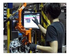
This standard functionality can be accomplished without any PLC programming required. Ujigami interfaces directly with sensors, torque controllers and other equipment, the label printer and scanner to ensure that the operator:
