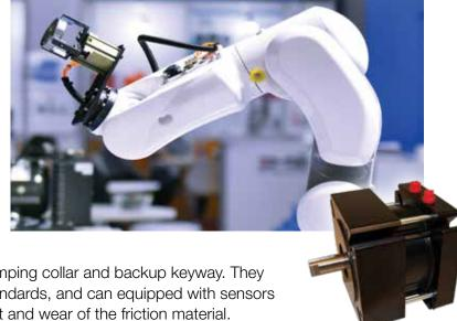
low-inertia brakes have an integral clamping collar and backup keyway. They produce zero-backlash, meet IP67 standards, and can equipped with sensors to detect engagement, disengagement and wear of the friction material.
