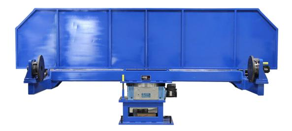
The Trunnions on either side allows for the fixtures to be oriented for ease of assembly into the holding fixture as well as the welding robots to get better access to either side of the panel.
