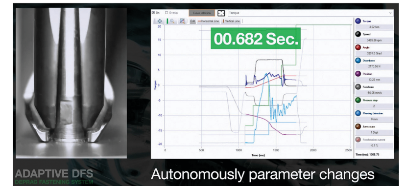
FIGURE [5] / Drive cycle timing flow-push screw
