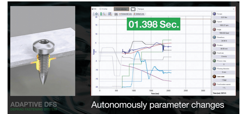
FIGURE [4] / Drive cycle timing flow-drill screw
