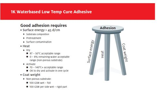
All applications are different, however, and require testing to evaluate the specific needs of the process to pass spec requirements. Two Henkel studies were designed to perform this type of evaluation.
