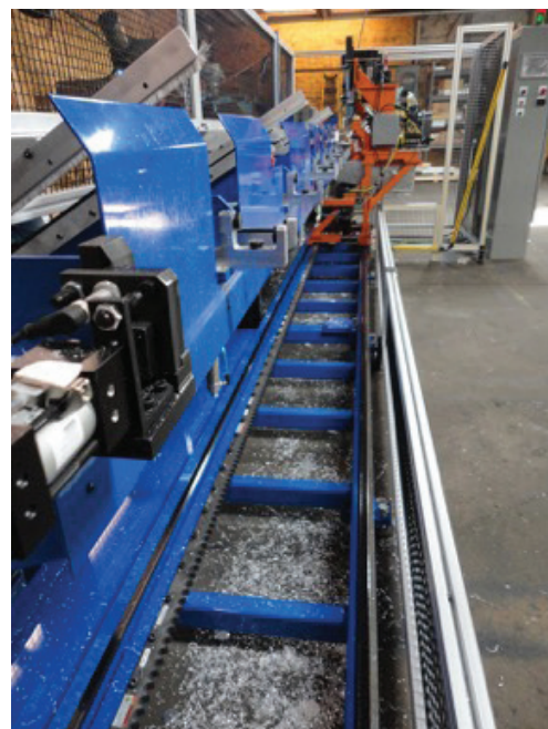
Lumco Manufacturing Co. integrated Nexen's Roller Pinion System into a custom machine for drilling and cutting aluminum. The Roller Pinion System moves a drill head along a 16-foot track at speeds of up to 2 feet per second.
