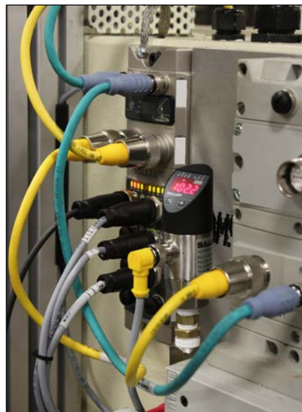
Figure 10: EtherNet/IP IO-Link Master with smart pressure sensor
