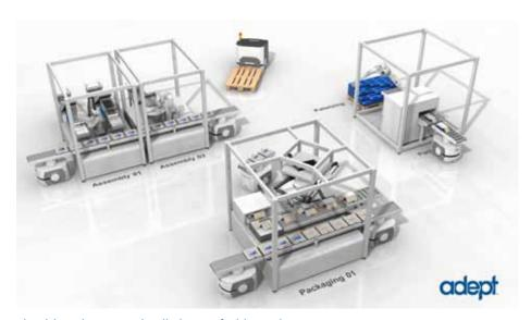
Flexible robotic workcells being fed by Adept Lynx AIV's.
