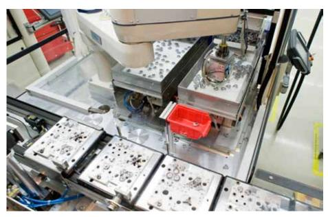
Electric Shavers being manufactured by an Adept Cobra robot from flexible feeders.
